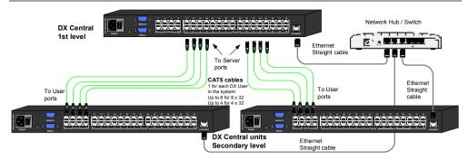
Figure 17 Cascaded DX Central units connected to a hub/switch
